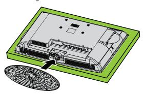
2 Secure the stand to the TV stand column using the six provided screws.
